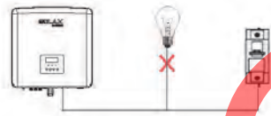
Figure: Wrong connection of load and inverter
